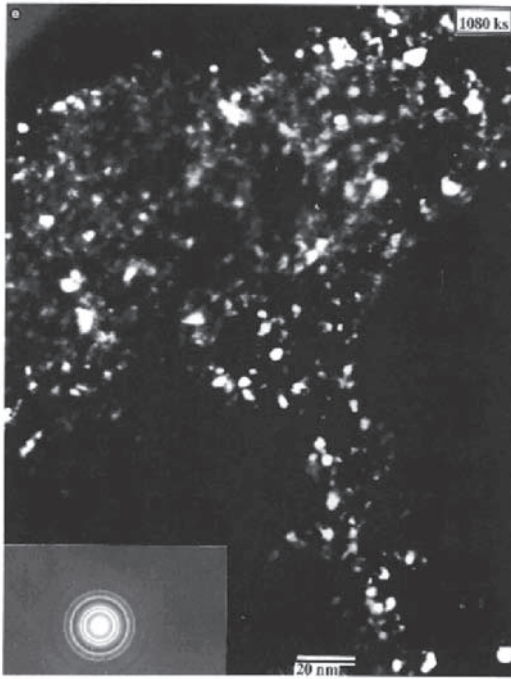
Figure 5.21. The DFI and corresponding SADP of the end product of \beta -SiC phase after 1080 ks of ball-milling time.
